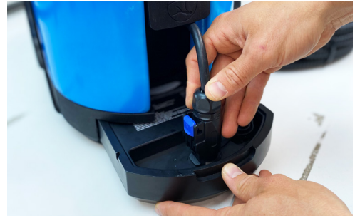
Power cable connector connected to Battery (No. 8)
