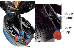
(2) Install screws into bottom of Nomad Mini. There are two sets of screwholes. The outside set is for the first DiveBoost, and the inner screwholes would be for a second DiveBoost.
